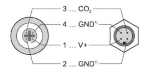
1) GND internally conected
