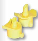
Replacement Saddles for Threaded Drinkers (VS205L / VS405L) – These saddles are a replacement for .875" square pipe (VS205L) or 1.1" square pipe (VS405L) that previously had threaded drinkers. The stems are slightly larger than the standard glued saddles so they can be glued into the existing threaded hole. These saddles accept any of our standard J-Lock Drinkers.
