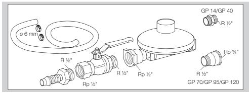
Pressure reducer, manual valve, hose (length = 2 m), 2 hose clamps, R 1/2" double nipple for GP 14/GP 40, R 1/2-Rp 1/2" reducing fitting for GP 70-GP 120, to connect the gas combination control CG to the gas supply, Order No.: N52600025
