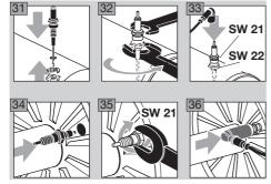
Ensure the electrodes are at the correct distance from one another and correctly positioned as regards the nozzle.
