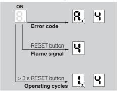
Error code: an error is displayed immediately in the form of an alternating letter and number indicating a warning or fault, see page 12 (Assistance in the event of malfunction).
