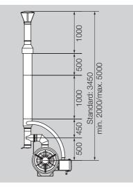
This example of application shows the chimney with the maximum installation length of 5 m.
