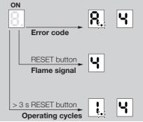
Error code: an error is displayed immediately in the form of an alternating letter and number indicating a warning or fault, see page 14 (Assistance in the event of malfunction).
