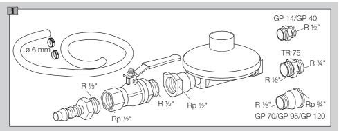
Pressure reducer, manual valve, hose (length = 2 m), 2 hose clamps, R  $\frac{1}{2}$ " double nipple for GP 14/GP 40, R  $\frac{1}{2}$ "/R  $\frac{3}{4}$ " double nipple for TR 75, R  $\frac{1}{2}$ " – Rp  $\frac{3}{4}$ " reducing fitting for GP 70 – GP 120, to connect the gas combination control CG to the gas supply, Order No.: N70000014.
